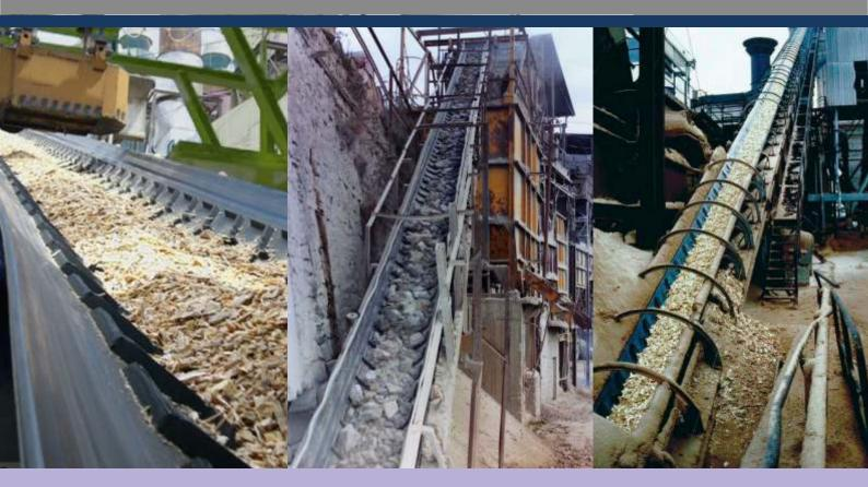
Space saving belts for Steep inclined and Vertical bulk material handling
