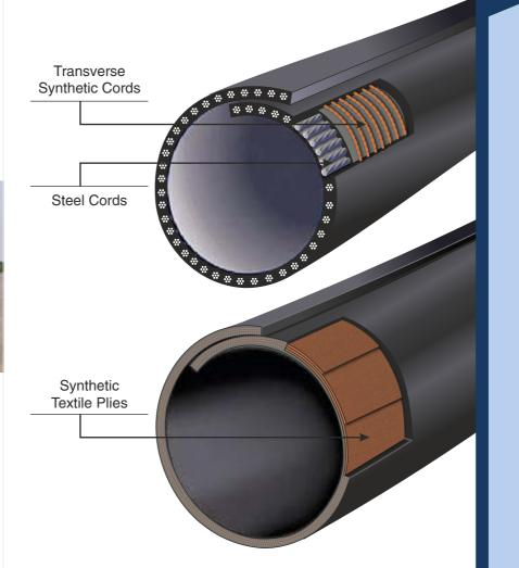
Forech has perfected the technology of supplying steel cord reinforced pipe conveyor belts and synthetic fabric reinforced pipe conveyor belts upto a maximum width of 2500 mm which translates to an inner diameter of 700 mm with adequate overlap. Various combinations are available depending on conveying path configurations.
